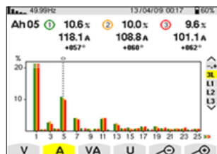
改造前电流谐波频谱 Current harmonic spectrum before modification
